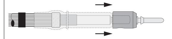
3 After tightening the contact, slide the cable reducer up until it butts against the contact.
