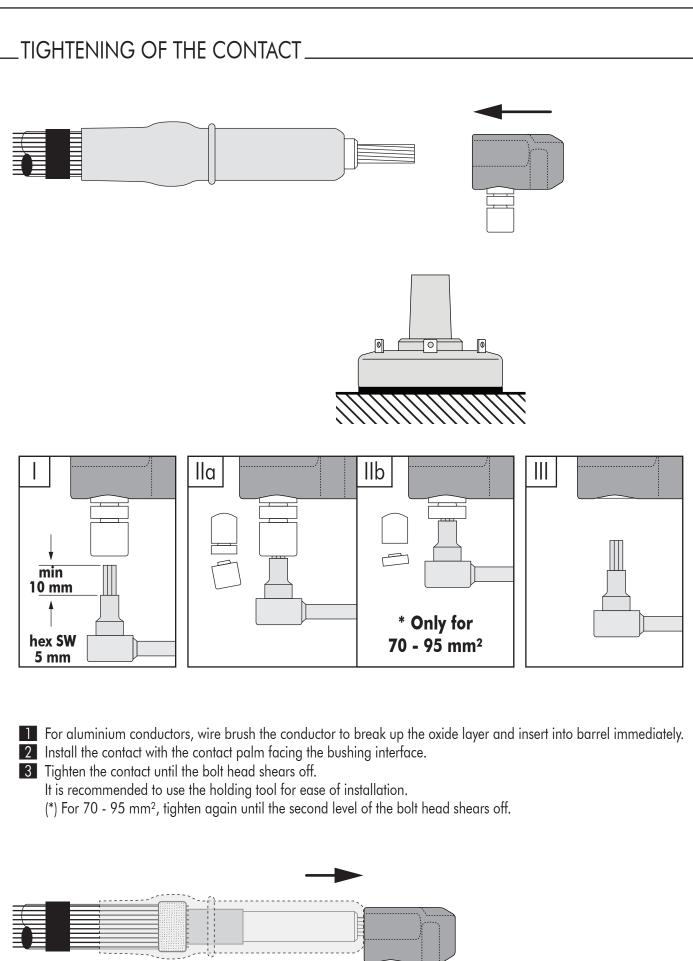
After tightening the contact, slide the cable reducer up until it butts against the contact.
