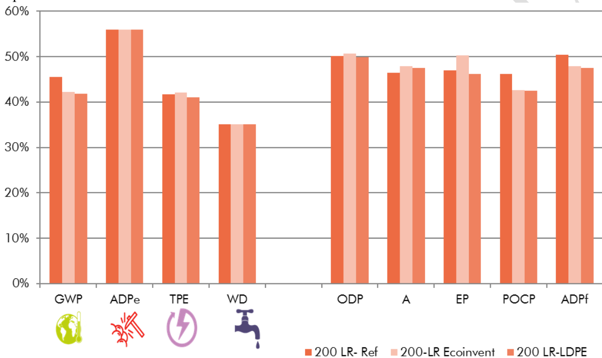
Figure 31: Sensitivity of the comparison of the manufacturing phase of 200-LR to the 158-LR depending on the type of LCI used to represent EPDM environmental impacts
